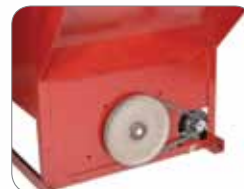
Motor driven auger with belt drive and removable guard.
