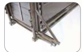
Alley panel rolls below platform out of the way
