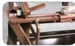
Gliding tailgate with simple one-handed manual release or air-operated release.
