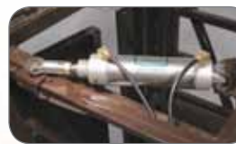
Single small bore super efficient air cylinder.
