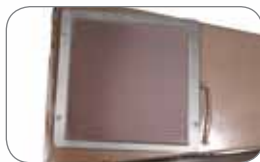
On-board solar panel for automatic battery charging.
